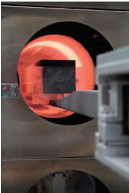
Energy-intensive: For electrical wafer orientation producers introduce phosphorus into the silicon at high temperatures in diffusion furnaces. (Photo: Q-Cells)
