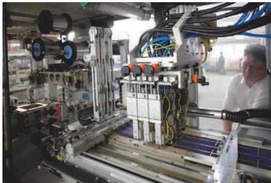
Not made for manual handling: Brazing individual solar cells to form strings is a hot topic: many brazing metals contain poisonous lead. (Photo: Aleo Solar)
