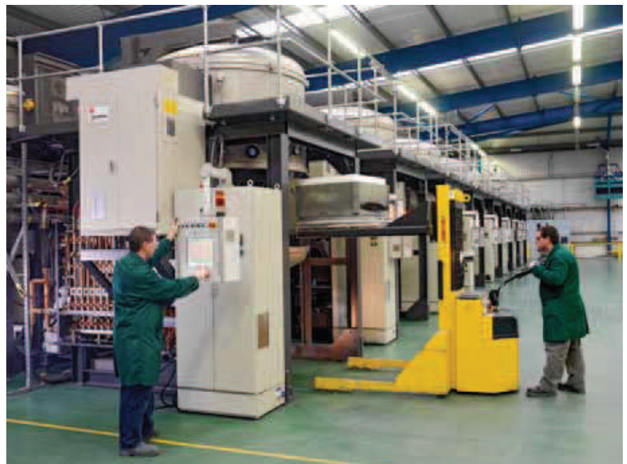
“Silicon bakery”: Employees at the silicon and wafer manufacturer PV Crystalox charge crystal-growing furnaces with raw silicon. Here the material is molten, freed from impurities, and then solidifies at a controlled rate. (Photo: PV Crystalox)
