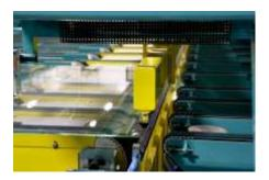
Fig. 2: After production the sheets are visually inspected and sized in a cutting line.
