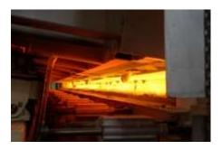
Fig. 1: The higher the temperature of the glass mixture in the melting unit the clearer the glass sheets produced.
