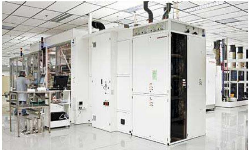
Checking the core machine: in a horizontal furnace wafers are processed further into cells. A Centrotherm technician checks its ready status. (Source: Centrotherm)
