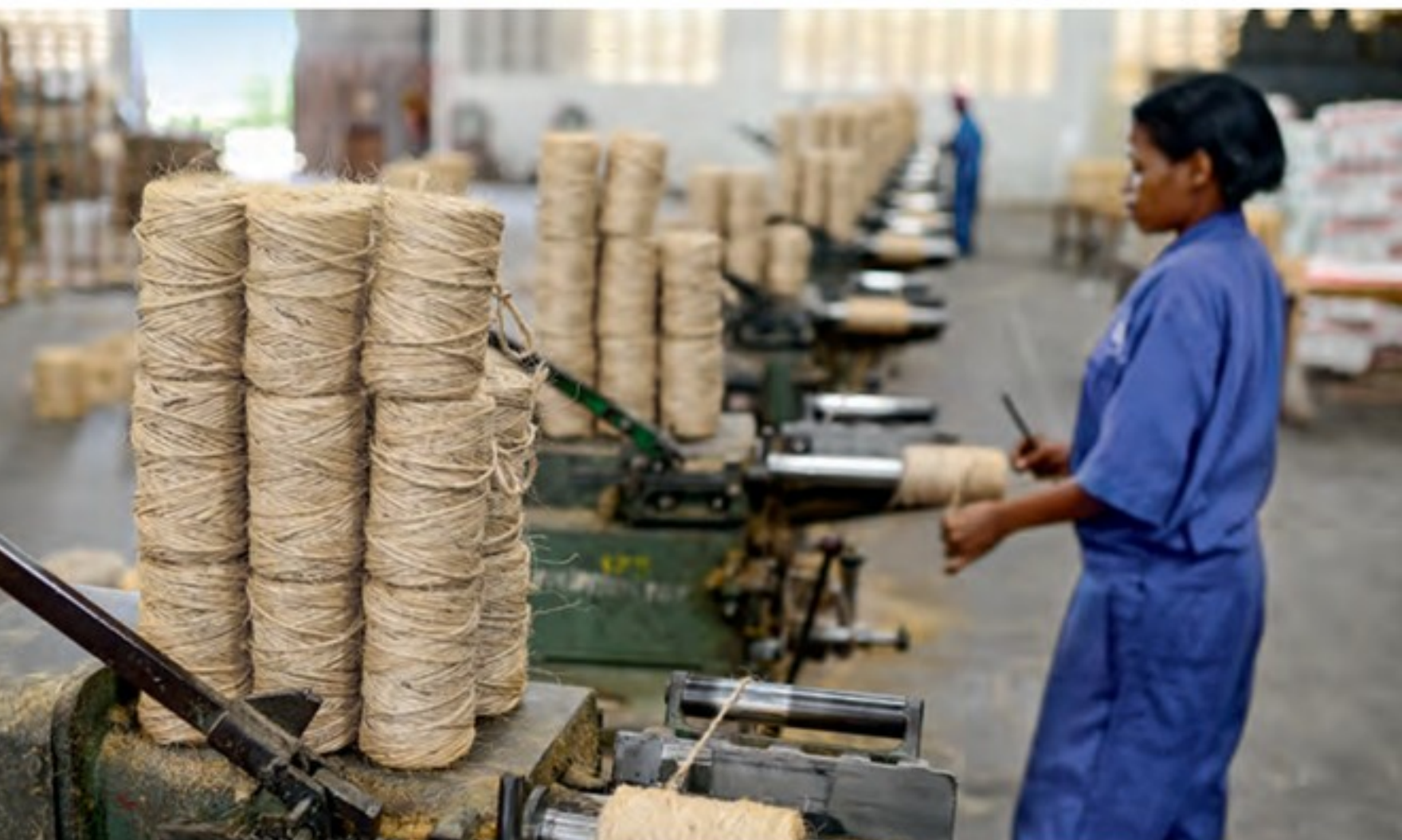
5 After combing out the residues, the fibre is pressed into large bales and transported for further processing. 6 View into the spinning work of Tancord (1998) Ltd. 7 Among other things sisal fibres can be turned into high-quality and environmentally-friendly twine and rope.
