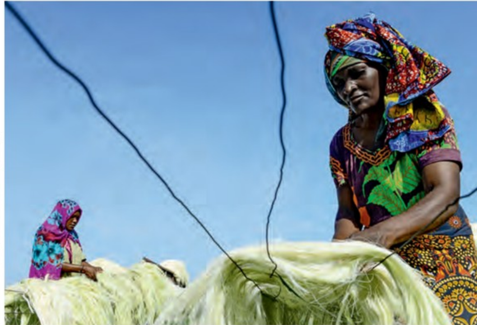
1 Freshly harvested sisal leaves are rolled into a machine that separates the fibres from the plant meat. 2 The machine squashes the sisal leaves, thereby separating the fibres from the other plant material. 3, 4 Workers are hanging up the separated fibres for drying on open-air racks.
