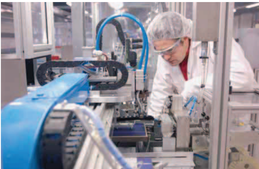
Spectators only: thanks to rapid technical advances by the solar machine manufacturers, the production process for solar cells is today a fully automatic one for many manufacturers. (Photo: Centrosolar)
